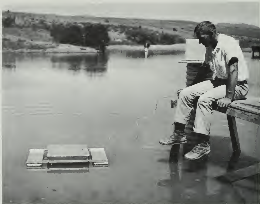
In studies in Arizona of evaporation losses from reservoirs, a hexadecanol raft applies a chemical film to the water surface to suppress evaporation.
